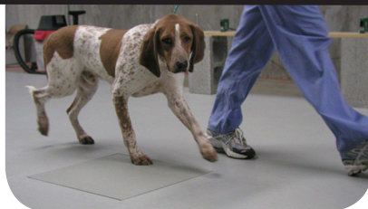
Force plate gait analysis for lameness measuring peak vertical force and vertical impulse.
